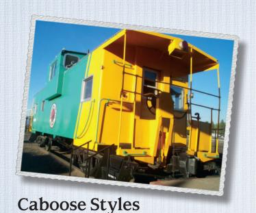
Cabooses came in different designs. This Northern Pacific Railway caboose is called a wide-vision cupola. Two other popular styles were the regular-width cupola and the bay window. Some cars were combination caboose-passenger cars used on mixed freight/passenger trains which operated primarily on branch lines.
